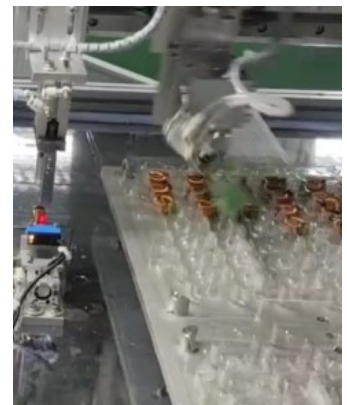
Auto universal test and unload to blister tray
